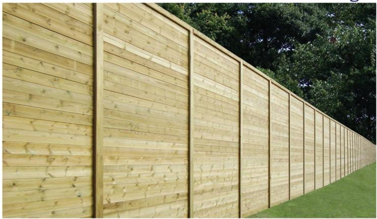
A lighter 20mm thick board than our other Jakoustic<sup>®</sup> barriers, maintaining the same 125mm cover face. Planed Tongue and Grooved boards with small chamfers which form a "V" join between boards. Suitable for installation where the required noise reduction is lower than that which would provided by the standard Jakoustic<sup>®</sup> noise barrier - or where a superficial mass of 10, 11 or 12kg/m<sup>2</sup> is specified.
