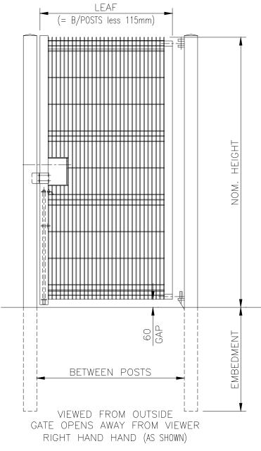
GATE SECURED USING PADLOCKABLE DROPBOLT & SLIDE LATCH (PADLOCKS NOT SUPPLIED)
