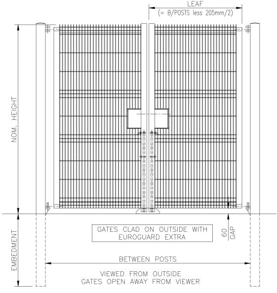
GATES SECURED USING PADLOCKABLE DROPBOLTS & SLIDE LATCH (PADLOCKS NOT SUPPLIED)
