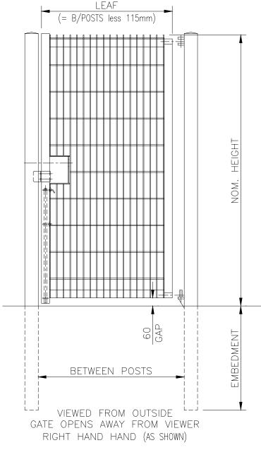
GATE SECURED USING PADLOCKABLE DROPBOLT & SLIDE LATCH (PADLOCKS NOT SUPPLIED) FOR OPTIONAL KEY LOCK REFER TO DRAWING J1/02111 FOR DETAILS.
