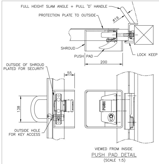
OPTION TO REMOVE HANDLE & KEY ACCESS & REPLACE WITH DUMMY BARREL TO PREVENT DEADLOCK OVERRIDE FOR PERMANENT FIRE ESCAPE ROUTES. \*PLEASE ADVISE WHEN PLACING ORDER\*
