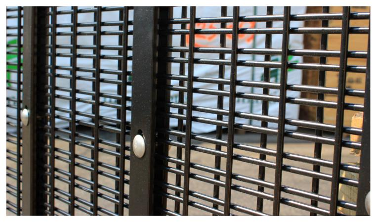
UHS Heavy Mesh SR3 has been designed and tested to withstand forced entry using tools which include battery power tools. The C5 (SR3) mesh system is constructed using 250mm wire double skinned mesh with clamp bars added at 250mm centres and anti tamper fixings.
