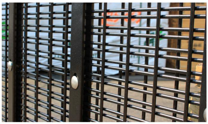
UHS Heavy Mesh SR3 has been designed and tested to withstand forced entry using tools which include battery power tools. The SR3 mesh system is constructed using double skinned mesh with clamp bars added at 250mm centres and anti tamper fixings.
