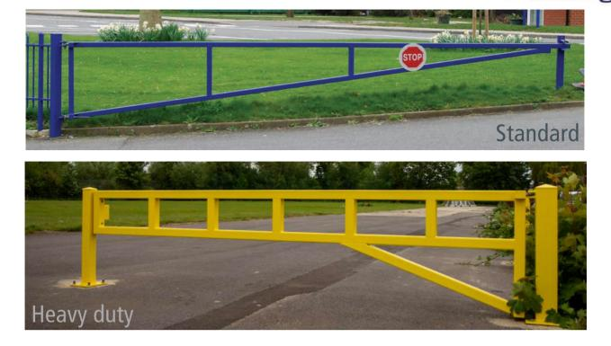
Our Warden Swing Barriers are available in both standard and heavy duty construction, making them suitable for a wide range of applications. Standard warden barriers are constructed using 60 x 60mm square hollow section (SHS), heavy duty warden barriers are constructed using 80 x 80mm SHS. Barriers come with anti-tamper hinges, and are padlockable in the open or closed position.
