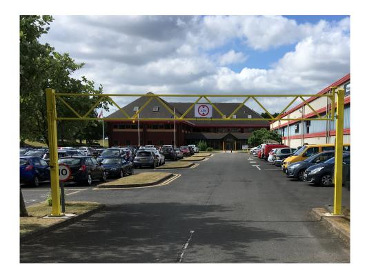
Height restriction barrier (with access) is made with square hollow section posts in a single and double configuration with a maximum road width of 10m. Designed to suit your specific road with and height requirement. Supplied galvanised as standard or powder coating as an optional extra. Padlockable in the open and closed positions.
