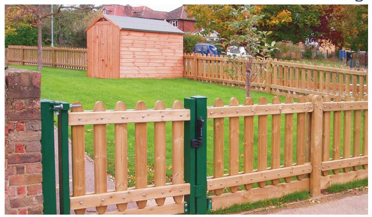
Designed to complement our Timber Playtime® and Metal Playtime® fencing, Playtime® gates conform to all current play area safety guidelines. Gates come complete with hinges that allow the gate to swing through an angle of 180° and 90° if a self closer is added. The hinges are fully adjustable with tamperproof screws and bolts.
