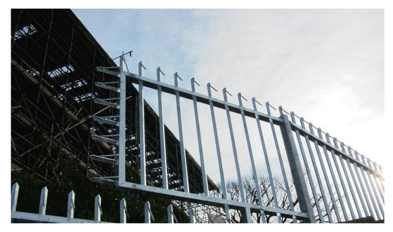
Barbican<sup>®</sup> Barbed Top panels are up to 3000mm high and have two horizontal hollow section rails 60 x 40mm (3 rails on 3000mm high). A 10mm round point bar is added to each pale downward pointing.
