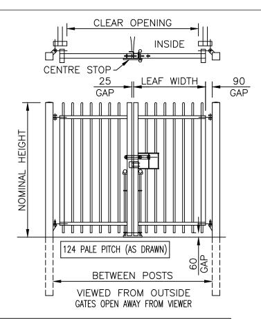
GATES SECURED USING DROPBOLTS & PADLOCKABLE SLIDE LATCH (PADLOCK NOT SUPPLIED) FOR OPTIONAL KEY LOCK REFER TO DRAWING J1/02111 FOR DETAILS.
