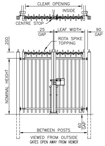
NOTES. ALL DIMENSIONS ARE IN mm (UNO) GAPS UNDER GATES & FENCING ARE NOMINAL DUE TO GROUND LEVELS. REFER TO DRAWING J1/04047 FOR GATE SIZE RANGE & DIMENSIONS.
