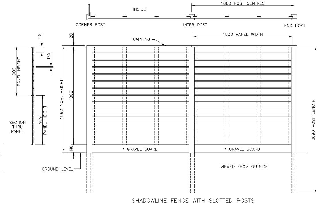
\* TO MEET THE CONDITIONS OF THE 25 YEAR JAKCURE GUARANTEE, GRAVEL BOARDS ARE REQUIRED WHERE PANELS ARE IN CONTACT WITH THE GROUND
