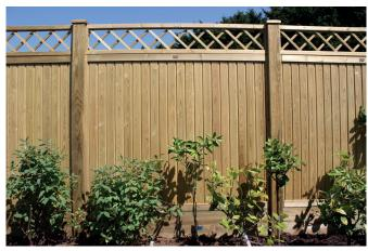
Tongue and Groove Effect panels are a mainstay of our premium panels range and available with a Level or Convex top. They feature a mortice and tenon jointed frame for extra strength while the infill is constructed using Tongue and Groove Effect boards, which incidentally match the infill used on our Courtyard gates.
