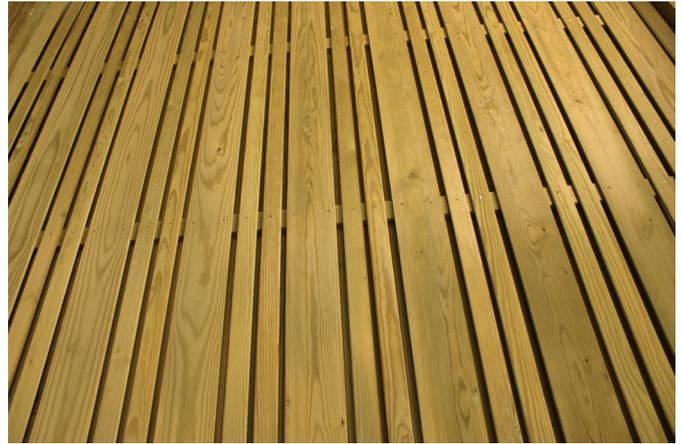
Combining wide and narrow timber pales, Urban is a contemporary panel with a distinctive design, ideal for a variety of applications. Mortice and tenoned frame for extra strength, these panels are planed all round for a smooth finish, with stainless steel fixings throughout to ensure a long life.
