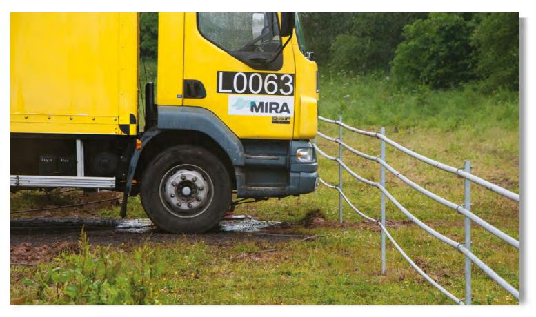
The Linebacker® PAS 68 Shallow Foundation is a cable type crash fence that has been successfully impact tested in accordance with BSI PAS 68:2010 to stop a 7.5 tonne vehicle travelling at 50 mph (80km/h). Its shallow foundations allow the fence system to be deployed in sites with utility congested substructures and underground services.
