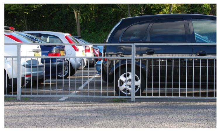
Specifically designed for highway applications, Jacksons Pedestrian Guardrail provides an effective roadside barrier for pedestrians while maintaining good visibility for motorists. The welded hollow tubular rail and solid pale construction is extremely strong and features a bolt-together design for ease of installation or replacement.
