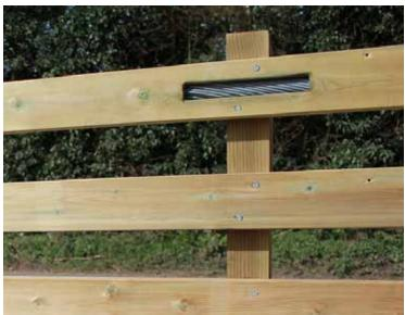
Linebacker<sup>®</sup> PNR features the PAS 68 certified and Secured by Design preferred Linebacker<sup>®</sup> crash fence system, concealed within a traditional timber post and rail fence design. Jacksons' Linebacker has been successfully impact tested in accordance with BSi PAS 68:2010, PAS 68 rating of PAS 68:2010 V/7500(N3)/80/90:7.3/21.4)
